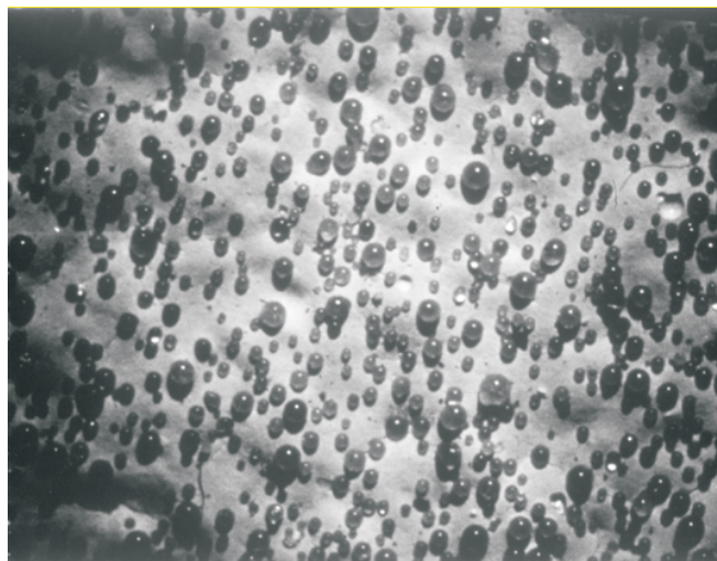
Figure 2.6 Improper bead embedment
