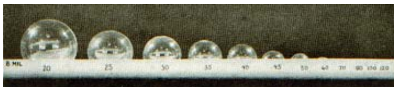
Figure 2.10 Beads in an 8 mil dry line
